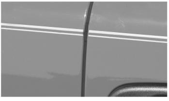
Trim stripe about 1/8" from all door edges, using light knife pressure when cutting. Trim ends of the stripe as desired.
