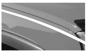
4. If necessary, lift the masking tape and reposition as needed if you don't lay it into a satisfactory position on the first attempt. Step back to view the overall placement of the tape. Adjust as needed.
