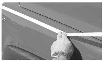
3. On the front fender, the stripe application may need to flow down at an angle toward the headlight. Align your masking tape with the top edge of the front fender, and lightly tack the masking tape into position.
