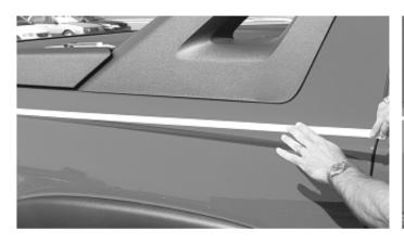
1. Determine placement of the pinstripe by using a line of masking tape as a guide. Start from the rear quarter panel and tack one end of the masking tape to the vehicle.
