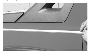
5. Lay the stripe along the bottom edge of the masking tape. Once in position, press firmly with your thumb or a squeegee along the entire stripe. Now peel back the clear premask at a 180° angle from the application surface.
